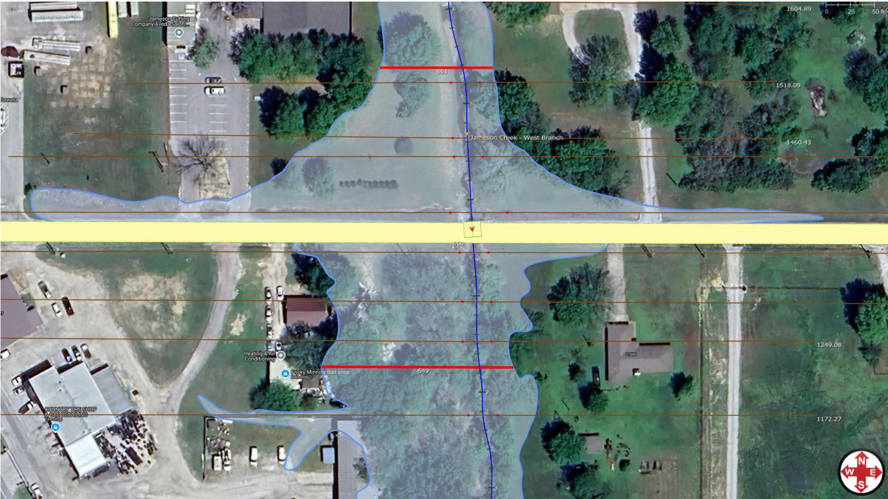
Exhibit 3.1 – Existing Spanned Bridge 1 Yr Storm Flood Elevations
