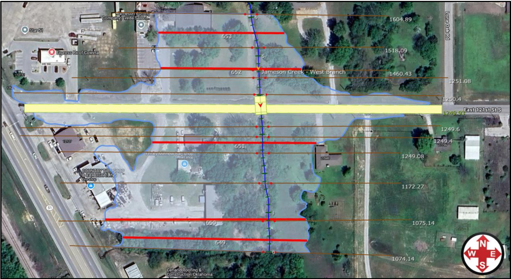
Exhibit 12.1 – Proposed RCB Culvert 25 Yr Storm Flood Elevations
